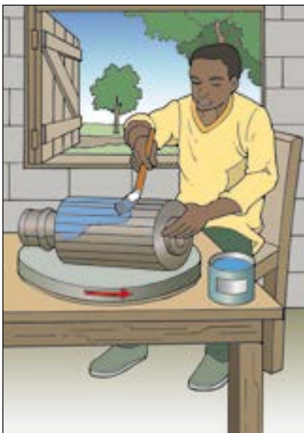
Figure 10c. Turntable for minimising the manual turning of heavy objects.
