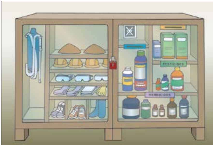
Figure 21c. Pesticides and personal protective equipment labelled and stored in a locked cabinet.
