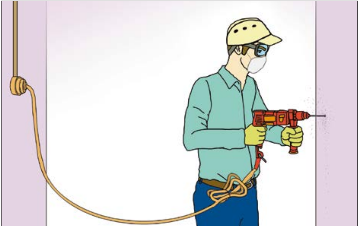
Figure 16a. Portable tools should be securely plugged into a socket which is away from water and out of a child's reach.
