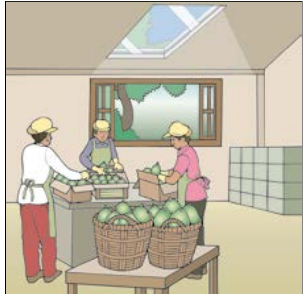
Figure 18b. Workstation benefiting from natural lighting due to the translucent panel in the ceiling and being near a window.
