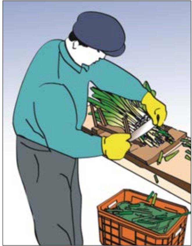
Figure 11b. Simple fixture for easy and safe cutting operations ensuring product consistency.
