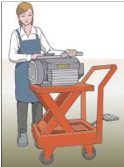
Figure 6b. Manually powered device for lifting heavy items to the working level.
