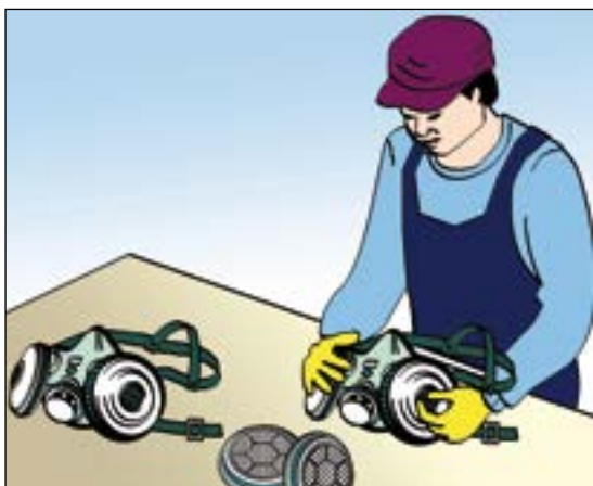
Figure 22d. Regular cleaning and maintenance (change of filters) for effective protection.
