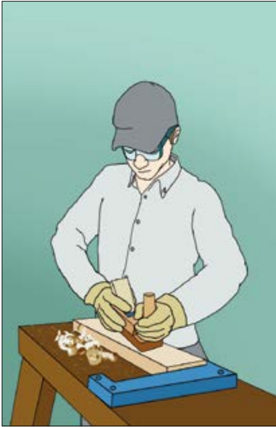
Figure 11a. Low-cost fixture made of pieces of wood, to hold workpieces for planing.
