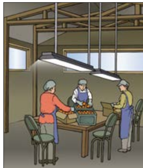
Figure 18d. Combined use of artificial light when daylight is insufficient.
