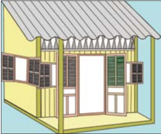
Figure 17a. Wide-open door and windows without obstacles, to increase the natural ventilation.
