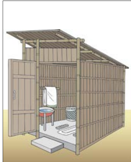
Figure 26b. Latrine-type toilet made from locally available materials.
