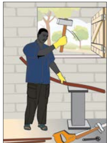
Figure 7c. Work height lower than elbow height when greater force is needed.
