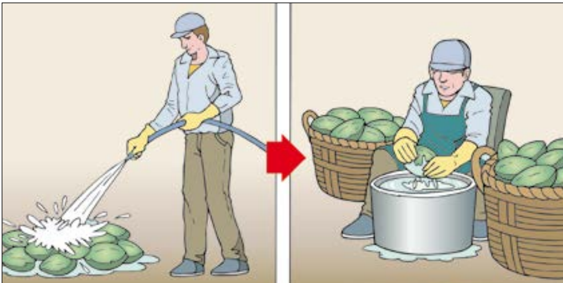
Figure 32b. Change of work process from continuous rinsing to batch rinsing saves water.
