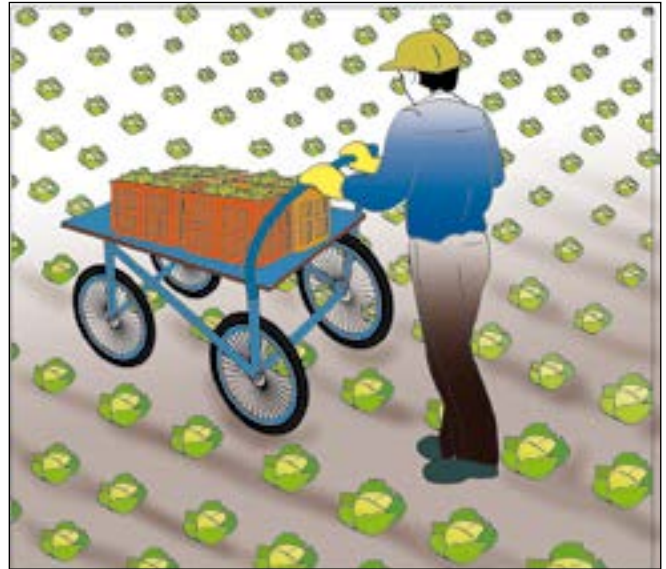
Figure 5b. Home-made cart made using bicycle wheels.
