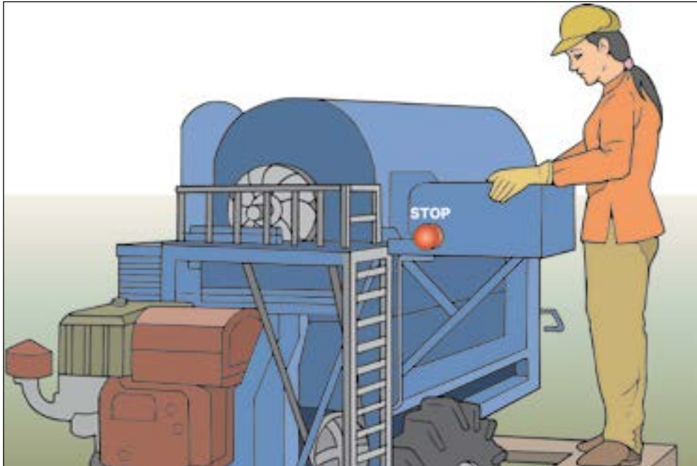
Figure 15a. Emergency stop, large and coloured red, within easy reach.
