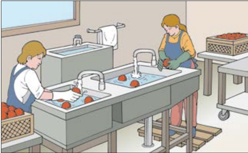
Figure 32a. Batch washing facility for cleaning products.
