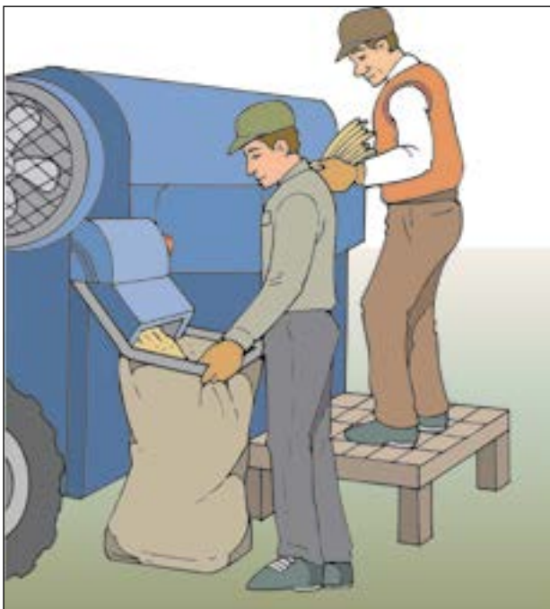
Figure 14b. Chute-type feeding device – using a platform to adjust working height for good working posture.
