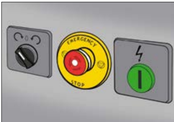
Figure 15b. Emergency stop on the control panel, large and coloured red with easy-to-read text.
