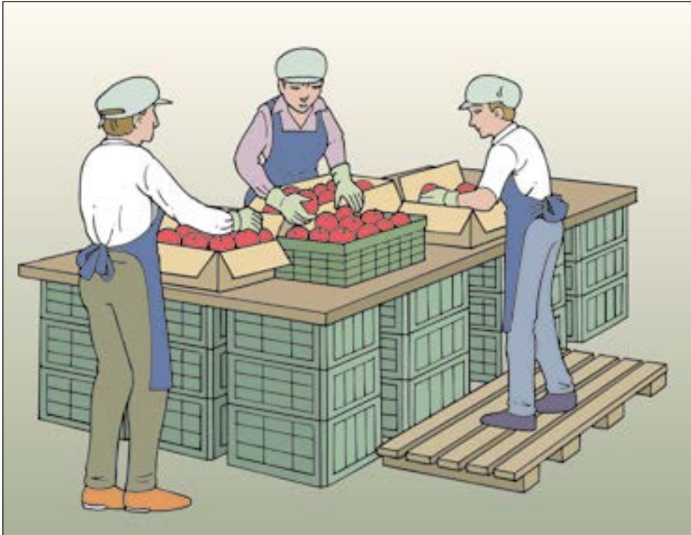
Figure 7a. A foot platform for a smaller person to adjust the work height to elbow level.
