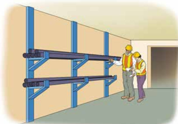
Figure 18.3. Multi-level racks keep materials in good order and help you keep the transport passageways and walkways clear and safe.
