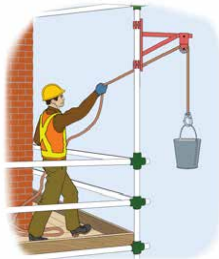
Figure 17.3. There are many examples of simple, low- cost devices to move heavy materials. Cooperation between workers is important for safe operation.
