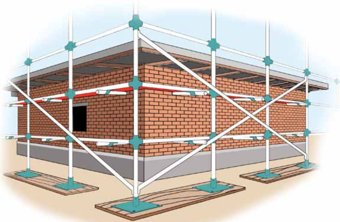
Figure 7.1. Secure the scaffolding to the building in enough places to prevent scaffold collapse.
