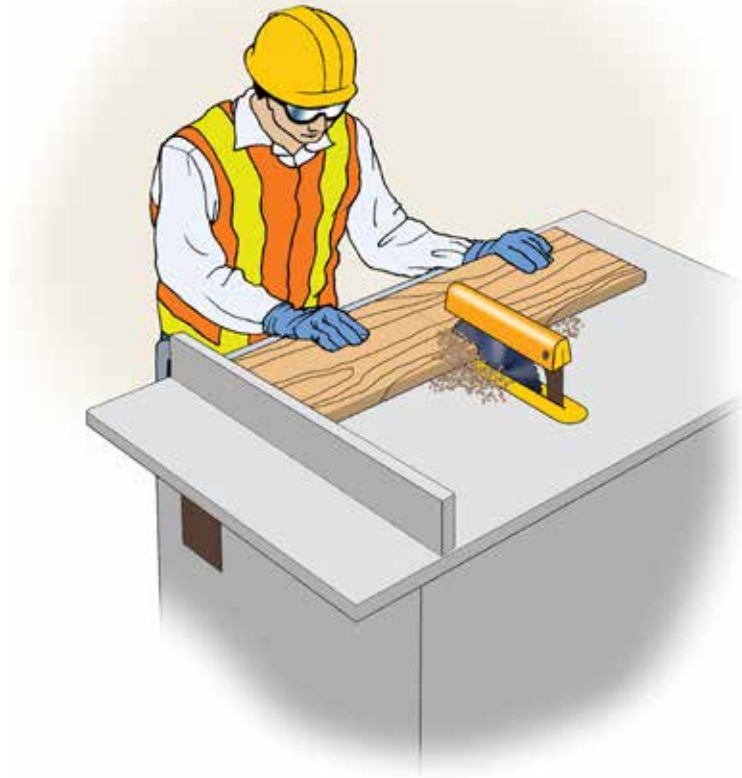
Figure 12.1. Attach proper guards to prevent access to dangerous moving parts.
