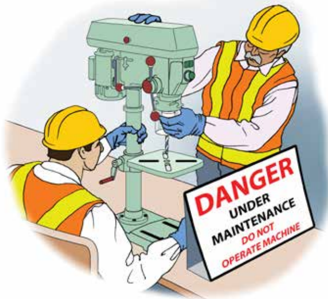
Figure 14.2. When maintaining or repairing a machine, make sure it is switched off and the electricity disconnected. Display a tag: "DANGER. UNDER MAINTENANCE. DO NOT OPERATE MACHINE."
