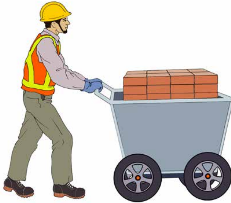
Figure 16.1. Use strong push carts with adequate wheels and holding points to carry heavy materials. Simple brakes should be used when carrying heavy loads, especially on ramps.
