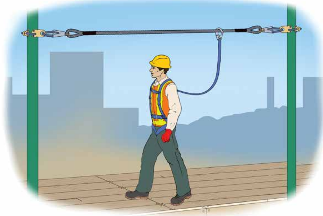
Figure 11.2. Use harnesses whenever performing work requiring additional protection, which is not – or not yet – covered by collective preventive measures against falls (e.g. guard-rails). Connect them to strong support systems (anchors, horizontal lifelines, etc.).
