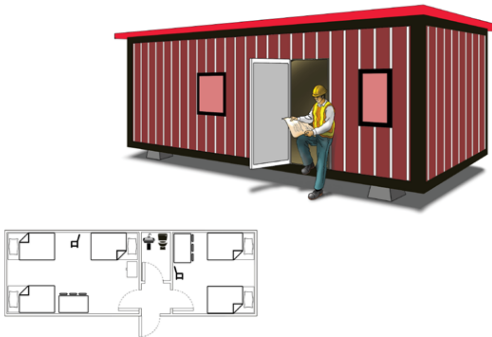
Figure 30.1. A typical example of a prefabricated accommodation facility for a construction site, including an example of an internal layout. It includes a sanitary facility for night use, but no showers.
