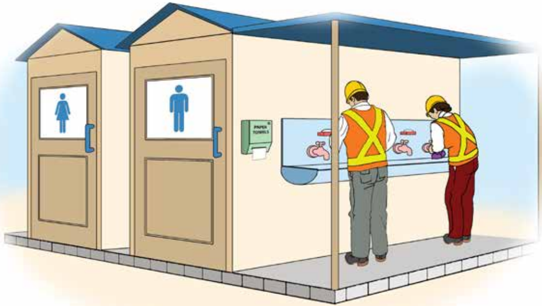
Figure 28.1. Provide separate hygienic toilets for women and men, as well as washing facilities, including paper towels.
