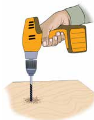
Figure 15.5. Battery-operated machines without a cable might be a safer option.
