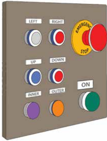
Figure 13.1. Attach clear labels for machine operations.
