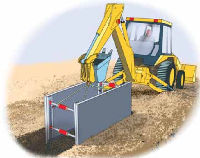
Figure 35.3. A safe installation of the trench box by machine.
