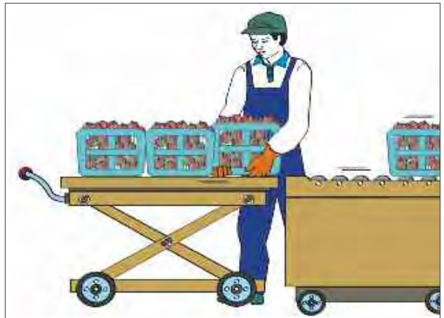
Figure 13b. Minimize height differences between the lift truck surface and the work table.
