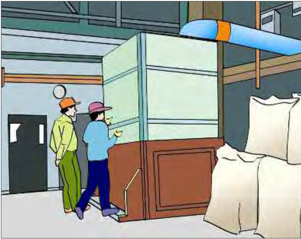
Figure 56a. Choose machines that have a good enclosure combined with an exhaust system.
