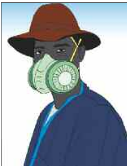
Figure 59d. The filters used for dust respirators are not effective for gases or vapours, and vice versa. Always use the correct types of respirator. Replace the filters in respirators frequently, in accordance with the suppliers' instructions.
