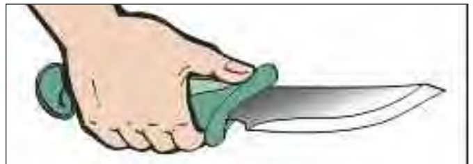
Figure 25c. Sharp tools might injure the fingers if the hand slips. Make sure that such tools are designed properly.
