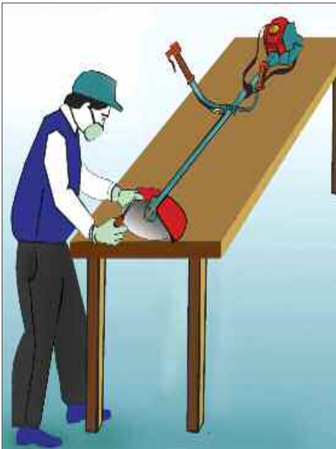
Figure 34c. Provide a stable work table of appropriate height for checking hand-held powered tools.
