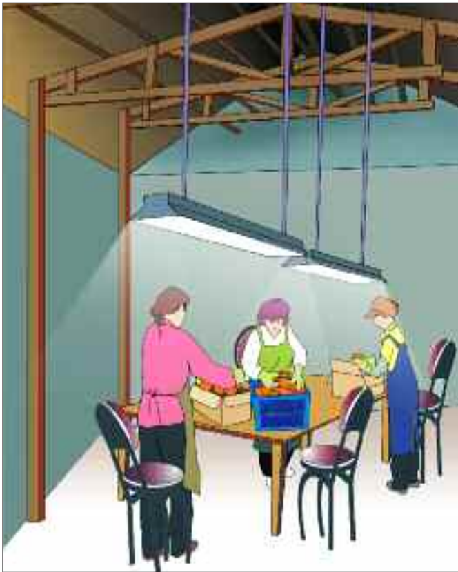
Figure 50a. Relocate lights to obtain sufficient lighting for precision or inspection work.
