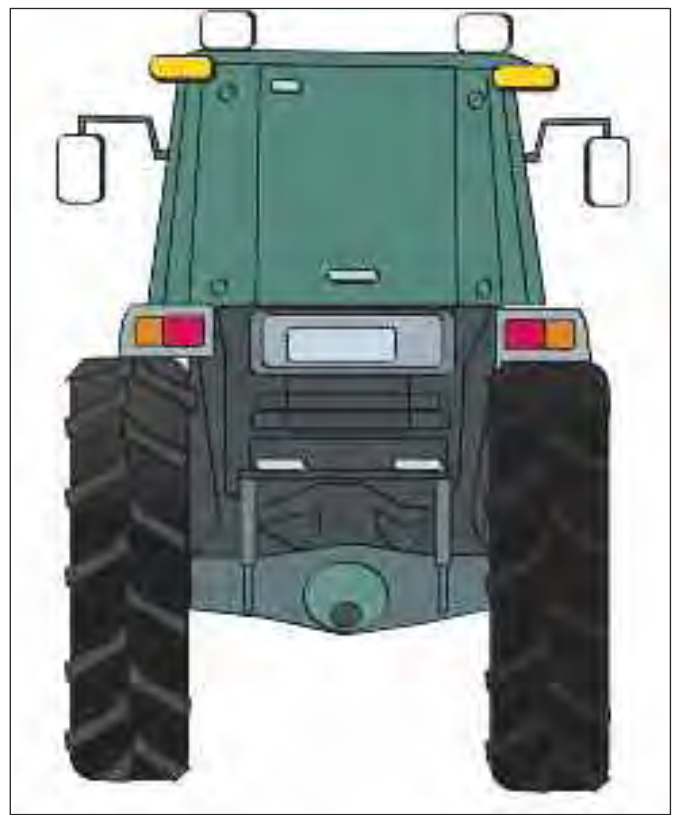
Figure 42b. Side mirrors on both sides of the vehicle, together with reflectors and additional lights.
