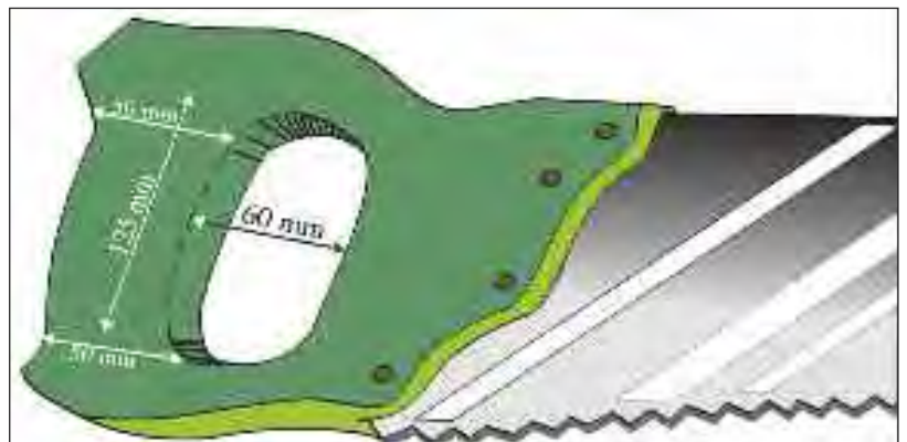
Figure 25e. The tool grip should be of the proper thickness, length and shape.
