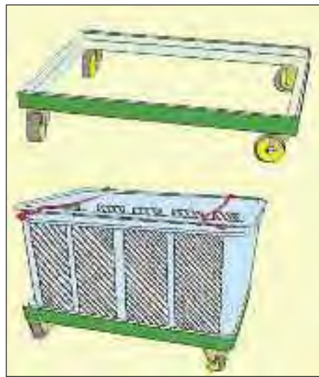
Figure 10b. Attach wheels to your containers.
