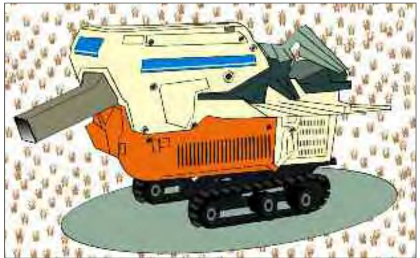
Figure 32a. Use wedges to fix machines with wheels, or use machines with caterpillar tracks.
