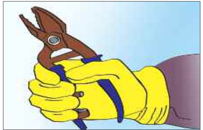
Figure 25b. The grips of tools should have the correct shape and adequate friction.
