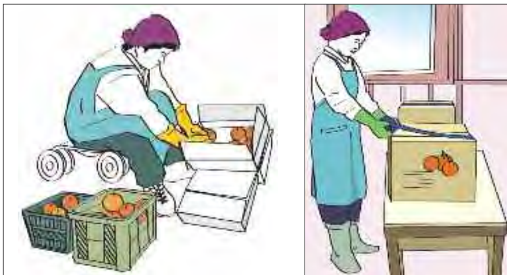
Figure 22c. Where possible, arrange standing work done at elbow level to replace low sitting postures.
