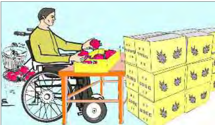
Figure 87b. Provide workstations suited for workers in wheelchairs and other workers with disabilities, so that they can work smoothly and comfortably.
