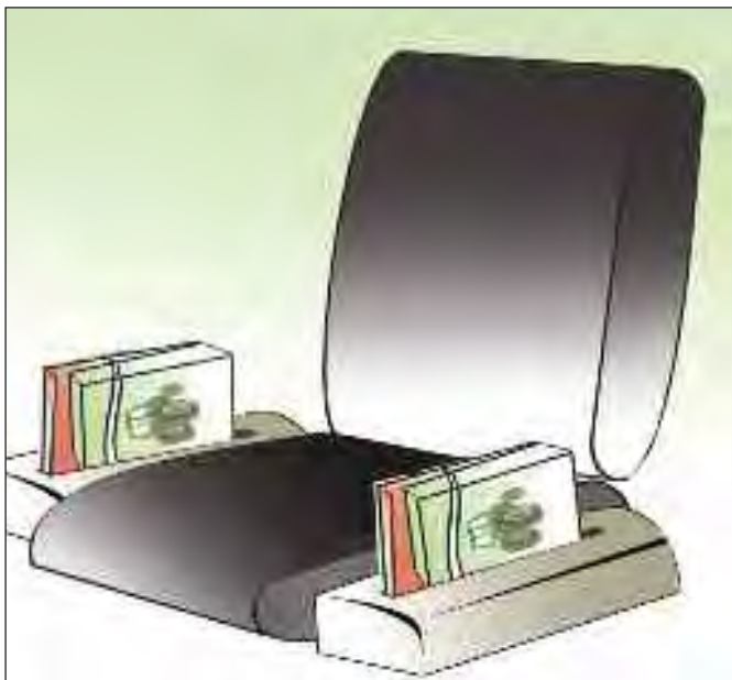
Figure 43b. Easy-to-read operation manuals and servicing instructions should be kept in the cabin and be available within easy reach of the driver.
