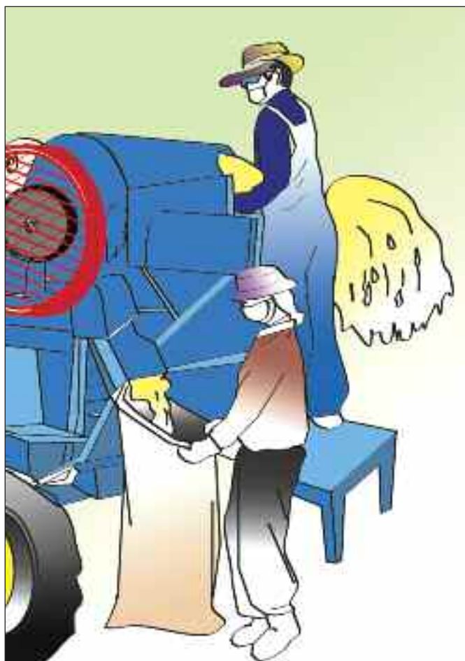
Figure 31a. Feeding device in the form of a conveyor which carries bundles of rice into the dangerous part of a threshing machine.
