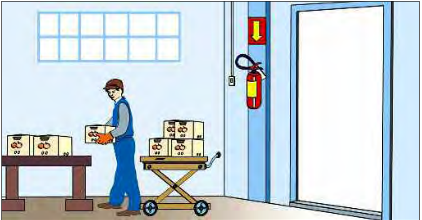
Figure 58a. Provide sufficient fire extinguishers at clearly designated places within easy reach from places where people work or live.
