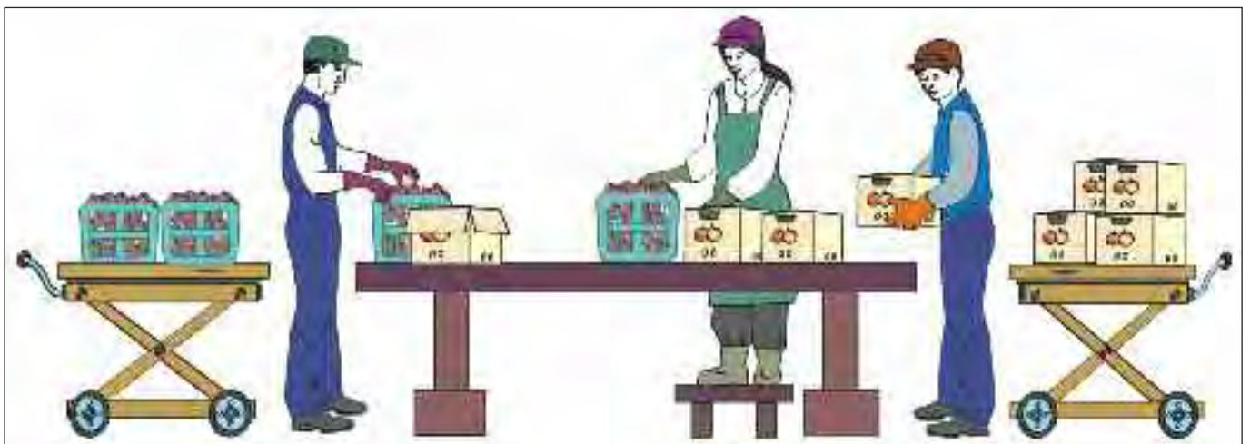
Figure 13c. Eliminate or minimize height differences between the work surfaces of different people. This minimizes lifting and lowering of items.
