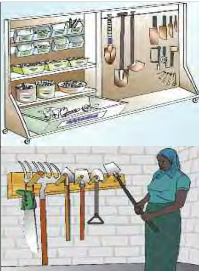
Figure 6b. Agricultural hand tools and personal protective equipment are placed tidily and in order on hangers and multi-level racks.
