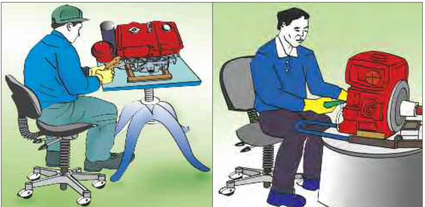
Figure 23c. A suitable sitting posture for work that requires care and concentration: table at or below elbow height; sturdy chair with backrest.
