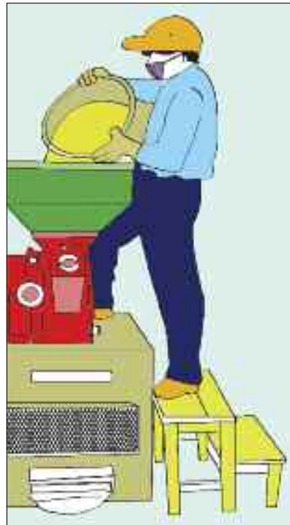
Figure 17d. Adjust the work height by using a stable foot platform corresponding to your elbow level.
