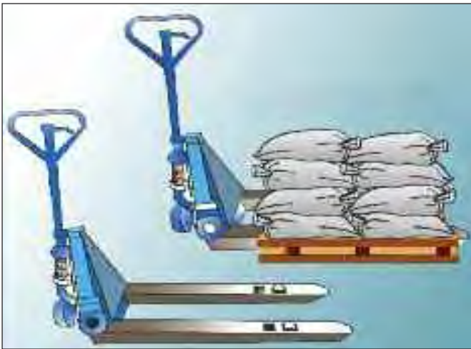
Figure 11a. A manually powered device to move pallets with heavy items.
