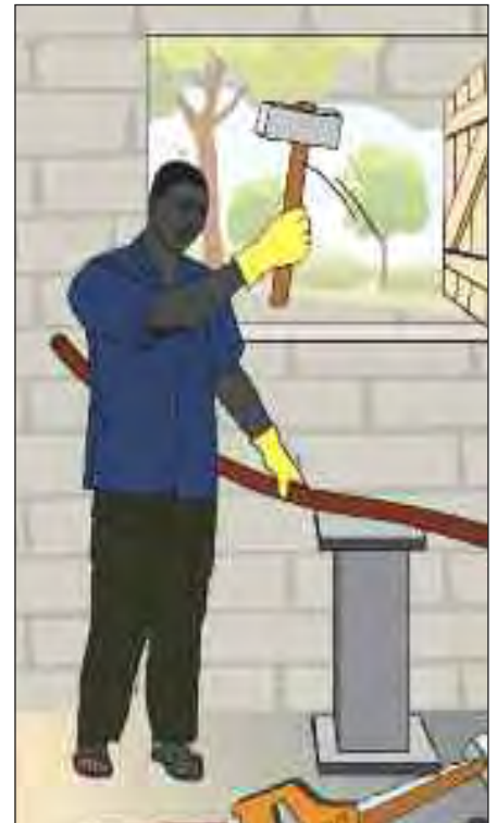
Figure 17e. When greater force is needed for work, choose a work height slightly lower than your elbow height.
