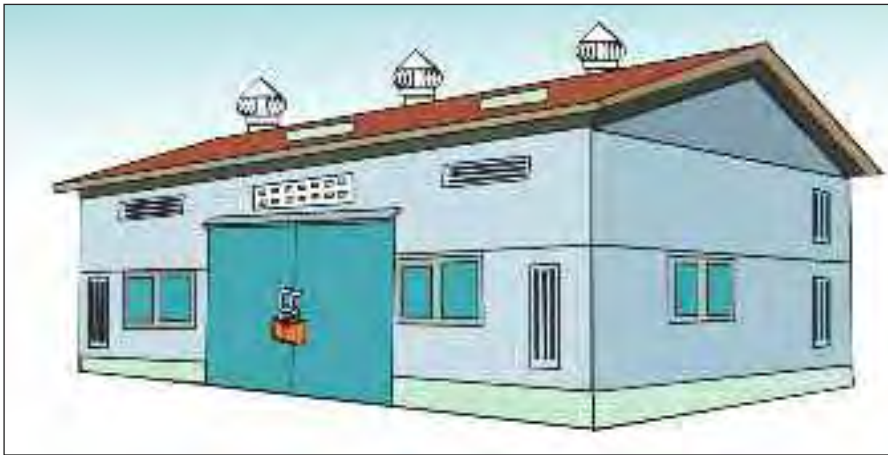
Figure 54b. Supply sufficient airflow when work is done inside a confined place to avoid accidents due to oxygen deficiency.
