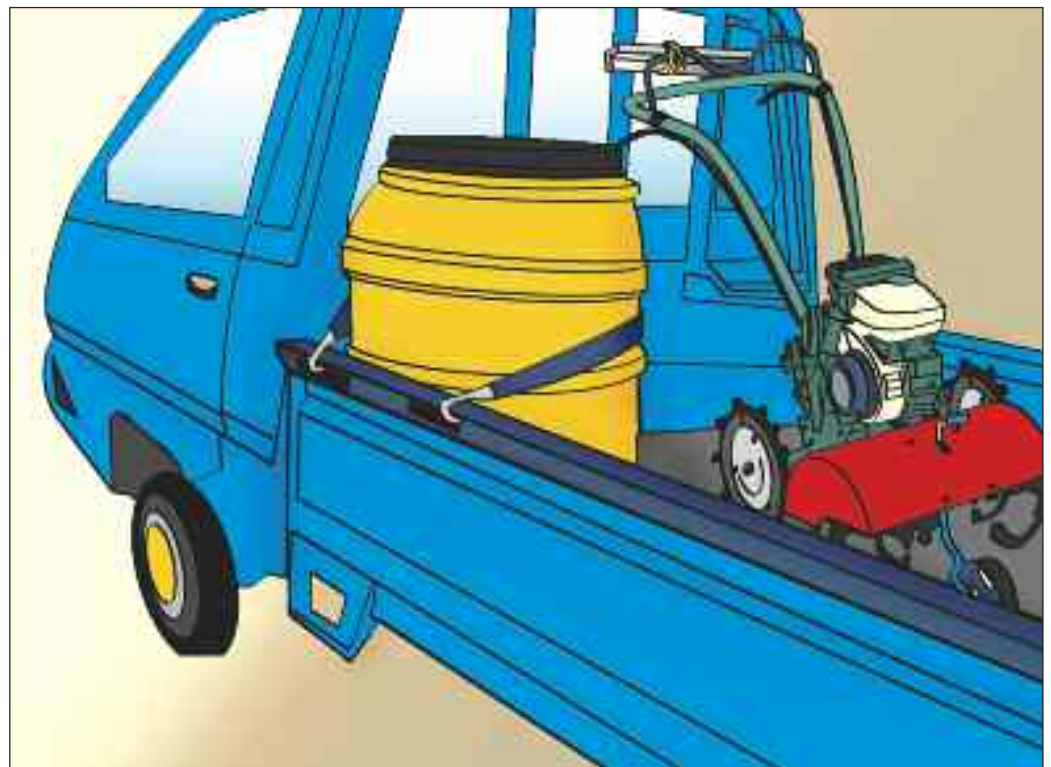
Figure 46c. Use proper rubber cords and special ropes for tying containers or machines of different shapes securely on the vehicle. Make sure that loads don't move during transport along bumpy routes.
