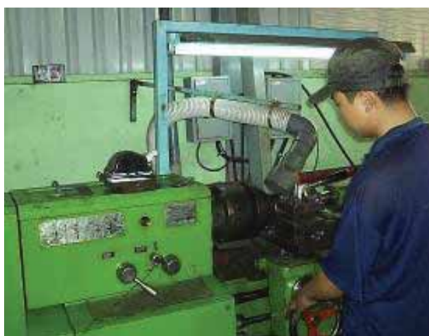
Simple local exhaust ventilation to absorb metal dust at a mechanical factory.
