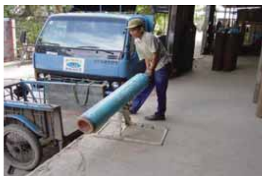
A simple rotating device to reduce the lifting of heavy material.
