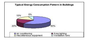
Typical break-up of energy consumption in a building is shown in Figure-1. In a typical building, air conditioning is the highest consumer of energy followed by
