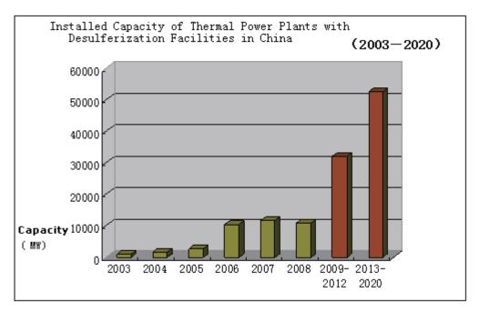
Figure 2-10: Coal-fired power plants with desulfurization facilities in China Data source: The State Development & Reform Commission and the State Electricity Regulatory Commission. Numbers for the 2003 to 2008 period is based on real data.
